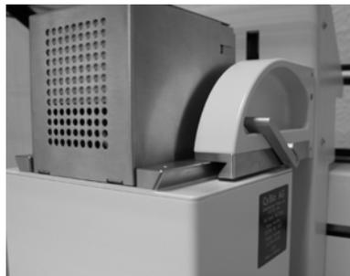
Fig. 15: Removal of pipetting head
