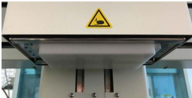
Fig. 17: Cover magazine (transport protection) attached
