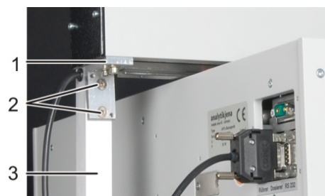
Fig. 44 Installing the stirring arm
