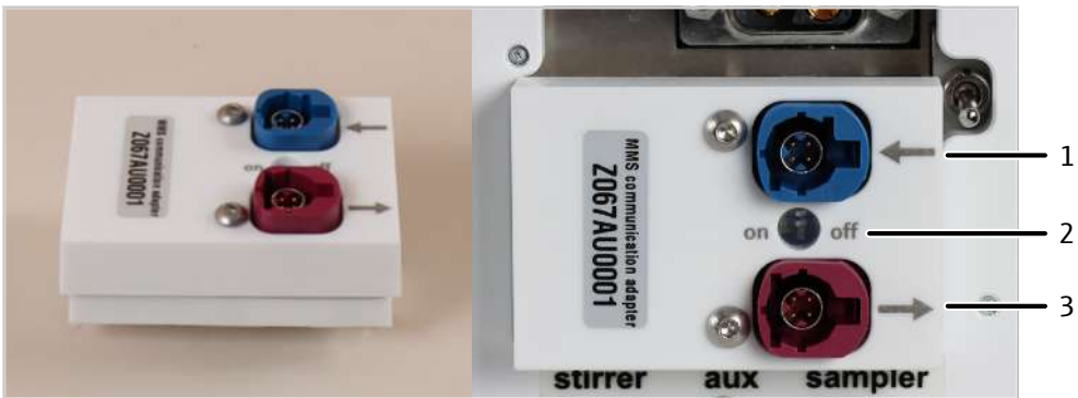
Fig. 14 Connector for connecting the analyzer (right: attached to the autosampler)
