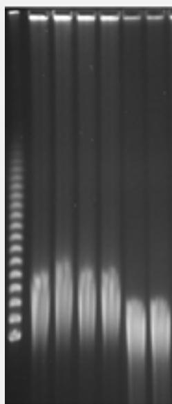
The quality of automatically extracted DNA from 200  $\mu$ L blood by InnuPure C16 *touch* on the basis of SmartExtraction was compared to the manual extraction via anion exchanger. The Rotaphor system (PFGE - Pulsed Field Gel Electrophoresis) shows the superior high-molecular weight of DNA extracts obtained by SmartExtraction.
