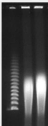
The genomic DNA from 10<sup>6</sup> NiH3T3 cells was extracted using the smart DNA prep (a) and InnuPure C16 *touch*. The Rotaphor system (PFGE - Pulsed Field Gel Electrophoresis) shows resulting high-molecular weight DNA of up to 450 kbp.
