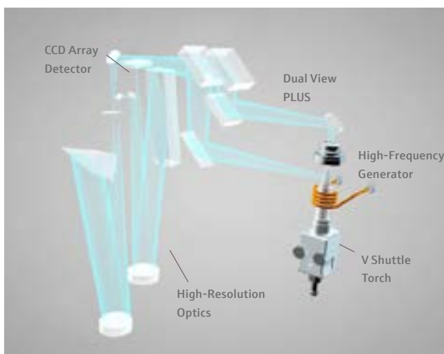
Scheme showing the main components of the PlasmaQuant 9100, including V Shuttle Torch, high-frequency generator, Dual View PLUS, and high-resolution optics.
