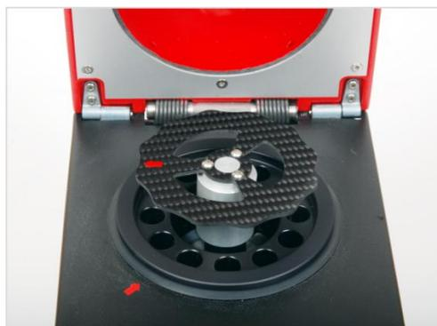
Fig. 8 Sample holder mounted to the SpeedMill PLUS
