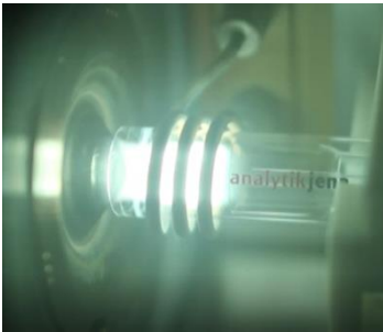
Figure 2: Hot plasma at 1.5 kW
