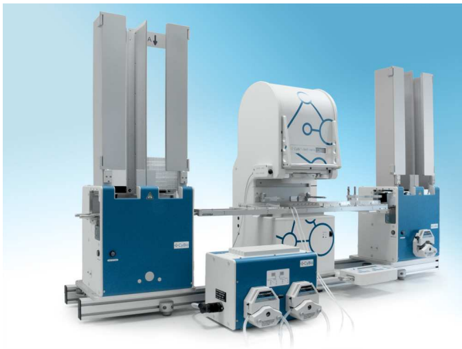
Figure 2: The CyBi®-Well vario with a 384/25 µL head and two stackers
