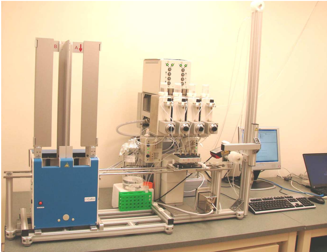
Figure 1: CyBio®-Drop 3D with four dispensing combs, one stacker and a barcode reader.
