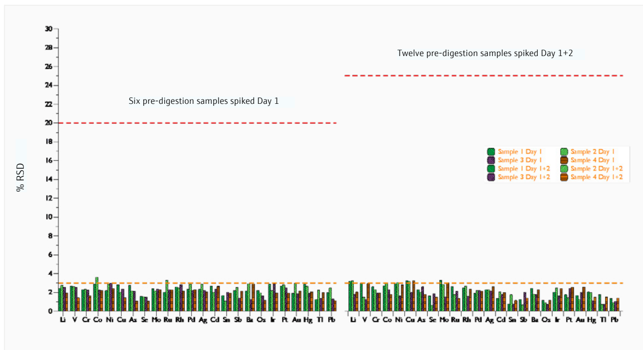
Figure 2: RSDs of six pre-digestion of all four samples analyzed in two different days. Criterion of 20% for day one and 25% for day-to-day stabilities accordingly to USP <232>
