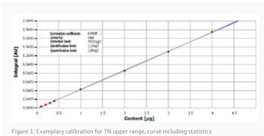
Figure 1: Exemplary calibration for TN upper range, curve including statistics
