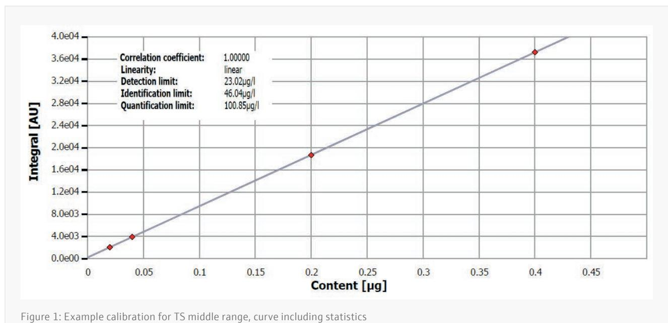
Figure 1: Example calibration for TS middle range, curve including statistics
