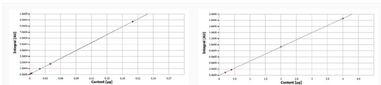
Figure 1 a–b: Multi-range calibration for the parameter TN, trace range (left) and high range (right)
