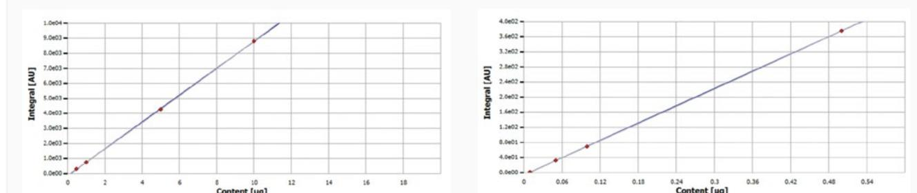
Figure 3 a–b: Multi-range calibration for the parameter TCl, trace range (left) and high range (right)
