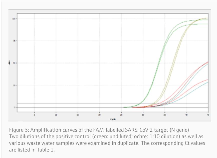
Figure 3: Amplification curves of the FAM-labelled SARS-CoV-2 target (N gene) Two dilutions of the positive control (green: undiluted; ochre: 1:10 dilution) as well as various waste water samples were examined in duplicate. The corresponding Ct values are listed in Table 1.
