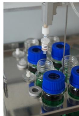
Figure 2: APU 28 SPE sample rack
